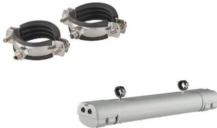
The Nemalux Pole Clamp Kit is designed to pole-mount any Nemalux Linear unit. The stainless-steel circular brackets are provided in a pair and easily screw to the back of the Linear unit, with adjustable side-bolts to open and clamp around a single pole. Kits to suit poles up to 62mm in diameter are available.
