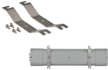
The Nemalux Ceiling Mount Kit is designed to mount to any flat surface, both ceiling and wall. Provided in a pair, two low-profile stainless-steel U brackets screw easily to the back of the Linear unit, then onto the chosen surface. 1000mm and 1500mm variants.
