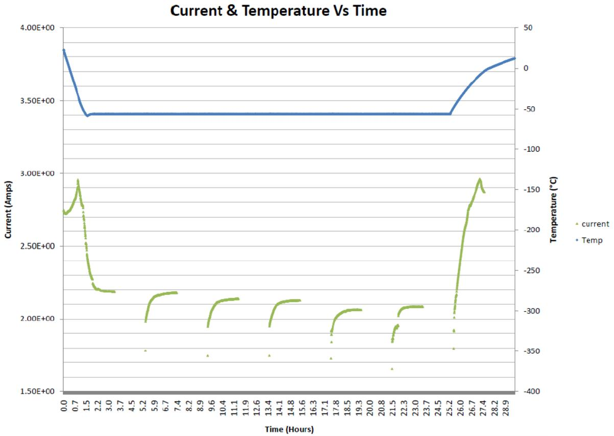
Figure 7. A plot of UUT current and temperature data collected vs time during the Nemalux part 1C test.
