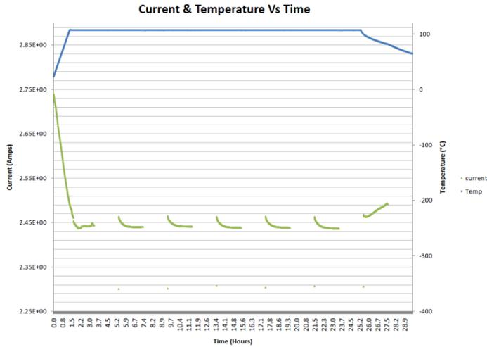
Figure 5. A plot of UUT current and temperature data collected vs time during the Nemalux part 1B test.
