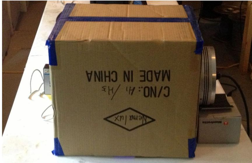
Figure 1: Spectrometer test jig. All corners sealed with opaque tape.
